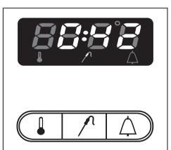
After a specific time the estimated time left until the cooking process has finished is shown in the oven display. From now on the actual temperature is no longer displayed, and cannot be called up.
